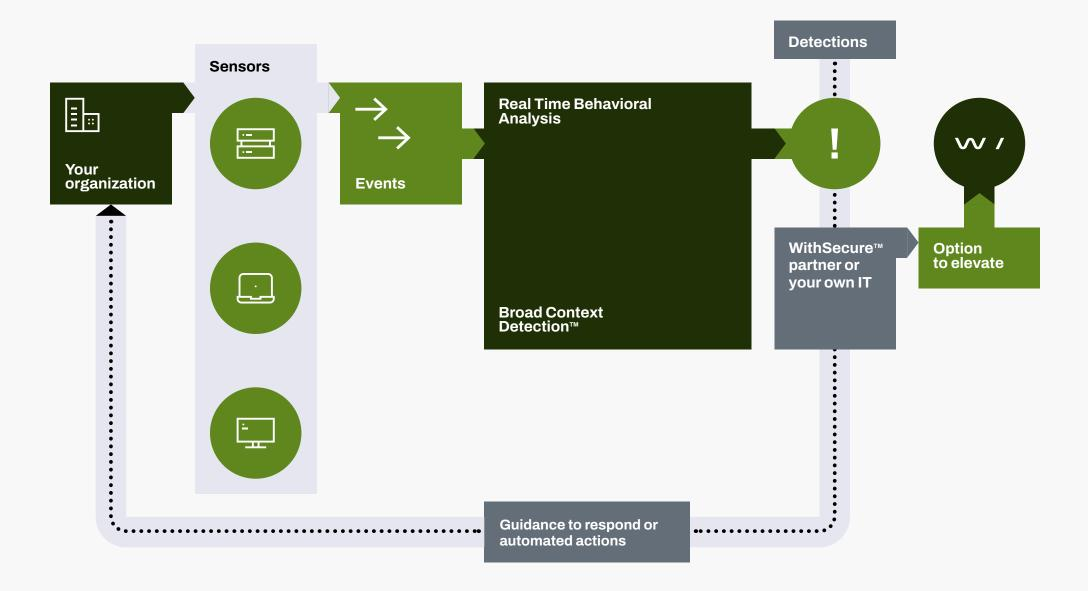
The figure describes on a high level how the WithSecure™ Elements Endpoint Detection and Response solution works:
